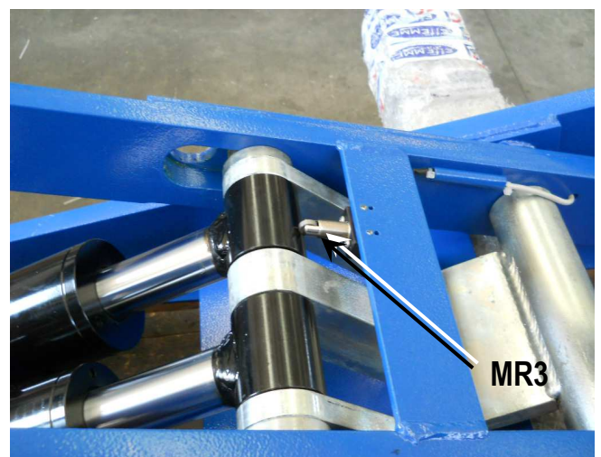
Pic. 24 P2 cylinder position sensing micro
