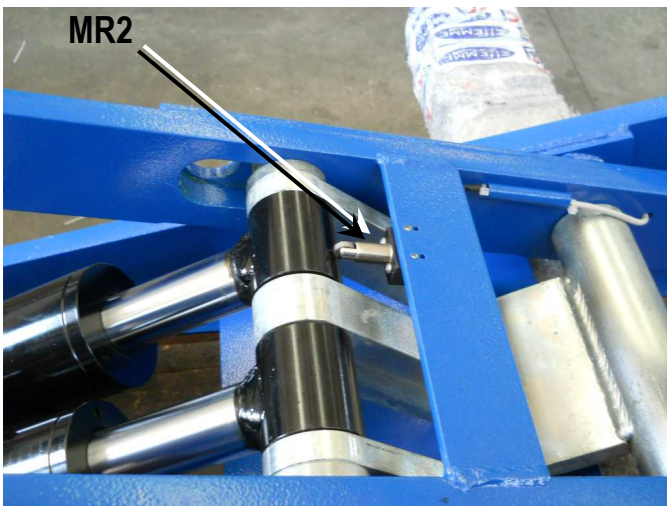
Pic. 23 P1 cylinder position sensing micro
